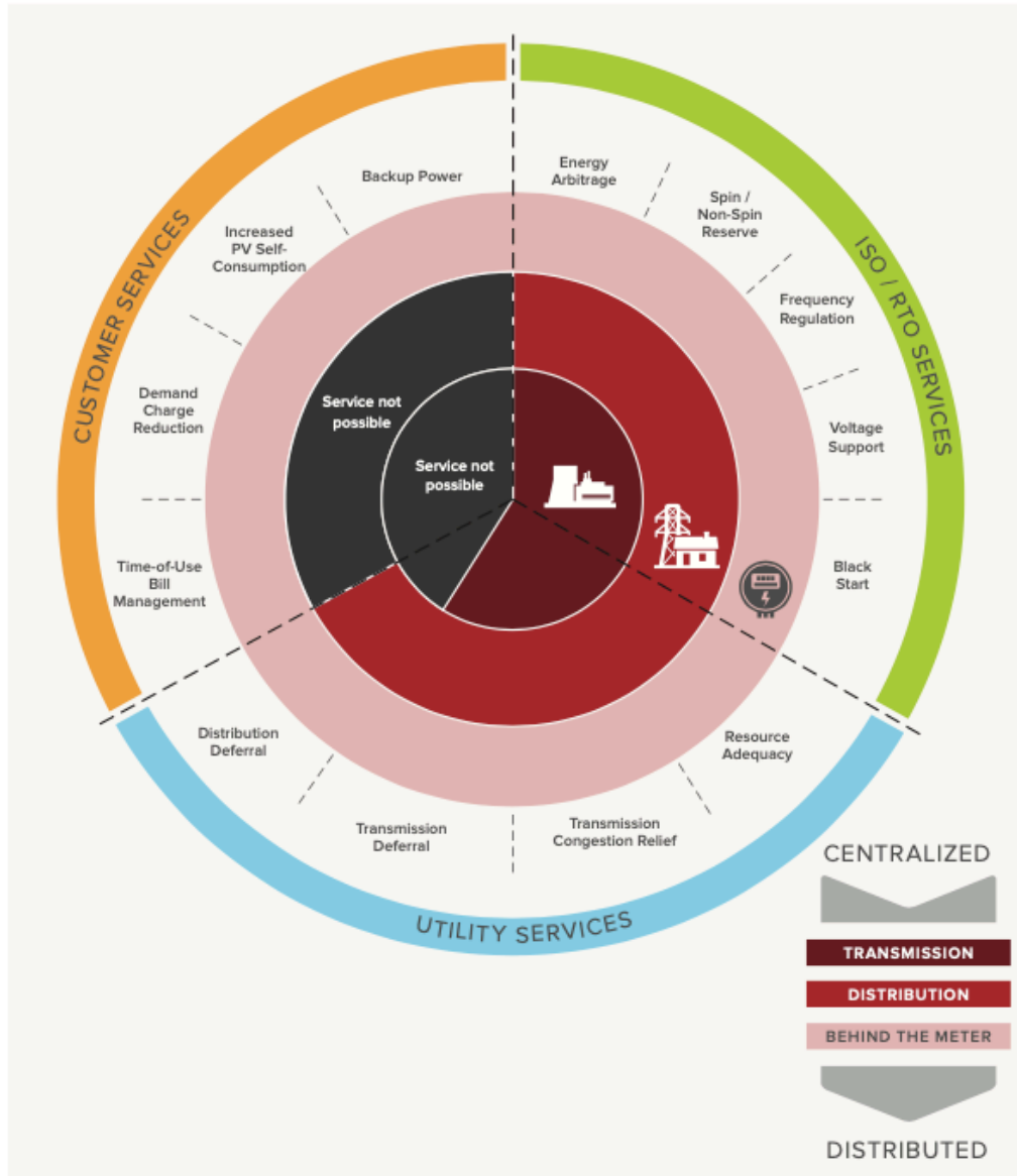
FIGURE 1: BATTERIES CAN PROVIDE UP TO 13 SERVICES TO THREE STAKEHOLDER GROUPS 22
