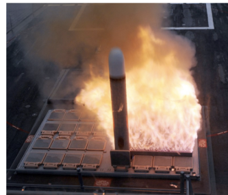
Mk. 41 launching a Tomohawk cruise missile. Source: U.S. Navy, Specialist 1 st Class Leah Stiles
